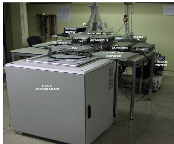
Fig. 5 : ACT validation test bench layout (left) and view (right)
